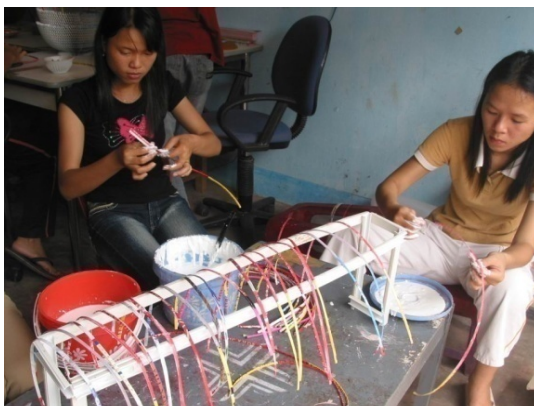
Gluing process of fold paper strips (Photo credit: Courtesy of MVH)
